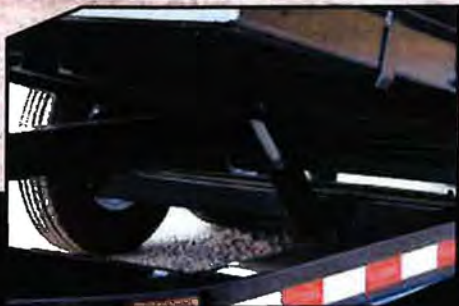
Cushion cylinder controls the deck when loading or unloading equipment.
