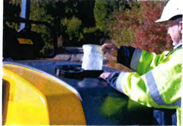
The water tank has a large opening for easy filling.
