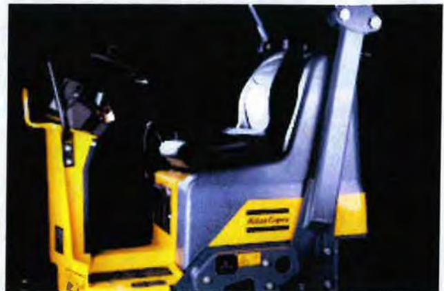
A spacious vibration-damped operator platform with comfort seat and dual forward/reverse levers for total operator comfort.
